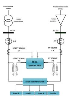
Fig.4. Single Line Diagram of SEMS
