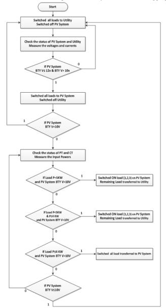
Fig.7. Algorithm of User Based Technique.
