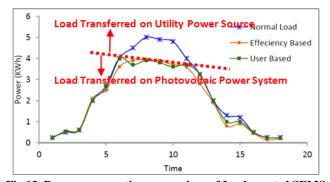
Fig.13. Power consumption comparison of Implemented SEMS
