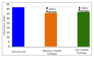
Fig.12. Experimental Result of Implemented SEMS
