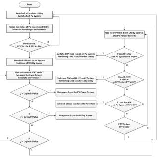
Fig.6. Algorithm of Efficiency Based Technique.
