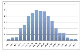
Fig.10. Hourly variations of power consumption w.r.t time in normal load control technique
