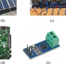
Fig.5. (a) Photovoltaic Power Generation System (b) 6 Photovoltaic panels (c) Electrical Contactor Relays for Load Transfer (d)Spartan 3AN FPGA starter kit (e) ACS 712 Hall
